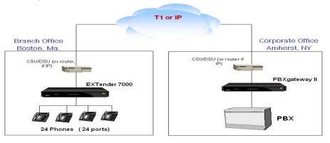
available in a managed IP environment (connects to the LAN via both 10/100 Base-T ports simultaneously)
